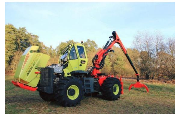
CAPOT MOTEUR, PROTECTION AVANT, RESERVOIR HYDRAULIQUE ET CABINE BASCULABLE HYDRAULIQUEMENT,
